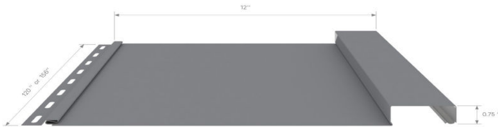
BOARD AND BATTEN - 12 in (304.8 mm) x 0.75 in (19.1 mm) x 120 or 156 in
