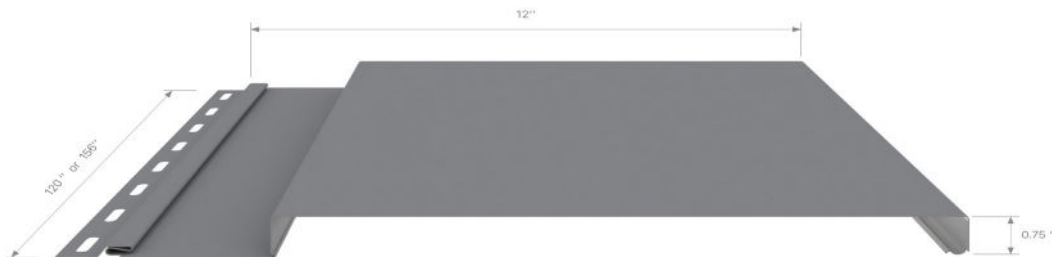
BOARD AND BATTEN INVERSÉ - 12 po (304.8 mm) x 0.75po (19.1 mm) x 120 ou 156 po
